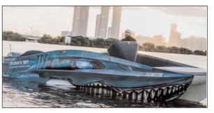
Cyberfin, a shark-shaped boat made from recycled ocean waste plastic, was completed in just six days and nine hours, highlighting the efficiency of this innovative technology. With dimensions of 10 meters in length, 2.1 meters in width, and 2.7 meters in height, it can accommodate up to 10 passengers and is officially registered with the Dubai Maritime City Authority (DMCA). **Fully 3D-printed boat**
