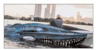
Cyberfin, a shark-shaped boat made from recycled ocean waste plastic, was completed in just six days and nine hours, highlighting the efficiency of this innovative technology. With dimensions of 10 meters in length, 2.1 meters in width, and 2.7 meters in height, it can accommodate up to 10 passengers and is officially registered with the Dubai Maritime City Authority (DMCA).
